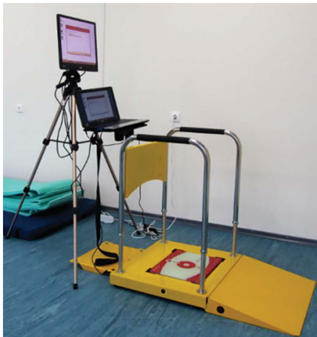
Figure 1. Force plate ST-150
